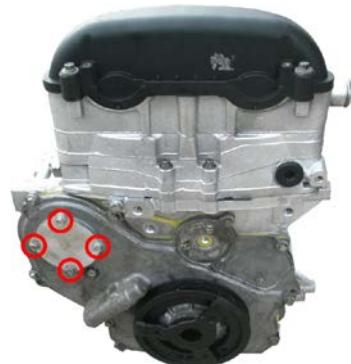
Attach the holding tool with 2 screws on the pump wheel and fix the tool onto the front cover, by using two original screws of the pump cover. Sprocket and timing chain will be held in the position and the pump can be removed.
