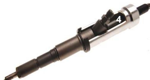
**Note:** Put the protective ring (2) below the puller (4).
