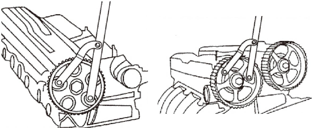
When loosening or tightening the screw, the counter holding tool must be rotated against the direction of the rotation of the screw.
