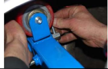
Roughly adjust cantilever using the 2-direction adjustment.
