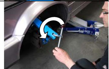
Move the flaring tool alternately from right to left and vice versa.
