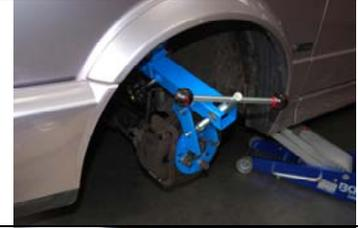
Loosen the flange roller with the tommy screws.
