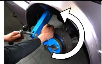
Check the pre-tensioning of the flange roller before each change of rotating direction and possibly re-tension.
